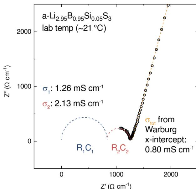
**Figure S14. Nyquist data for a-Li<sub>2.95</sub>B<sub>0.95</sub>Si<sub>0.05</sub>S<sub>3</sub> near room temperature.** The partially resolved semi-circular features suggests the presence of at least two RC circuit elements.
