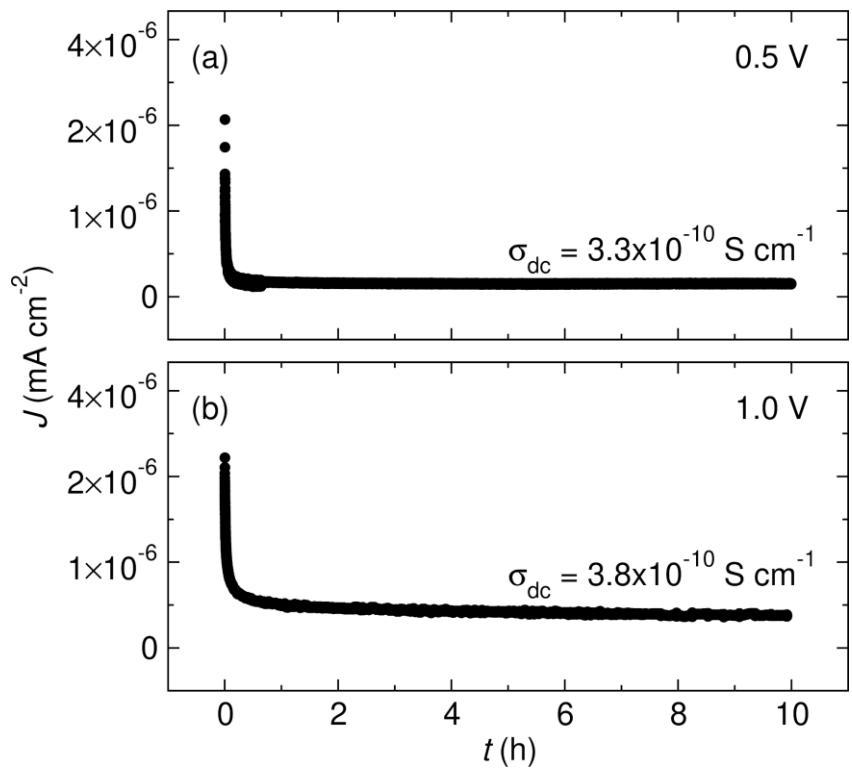
**Figure S18. DC polarization of an  $\text{Au}/\text{a}-\text{Li}_{2.95}\text{B}_{0.95}\text{Si}_{0.05}\text{S}_3/\text{Au}$  cell.** Measurements were done at  $25^\circ\text{C}$  with applied voltages of (a)  $0.5 \text{ V}$  and (b)  $1.0 \text{ V}$ .
