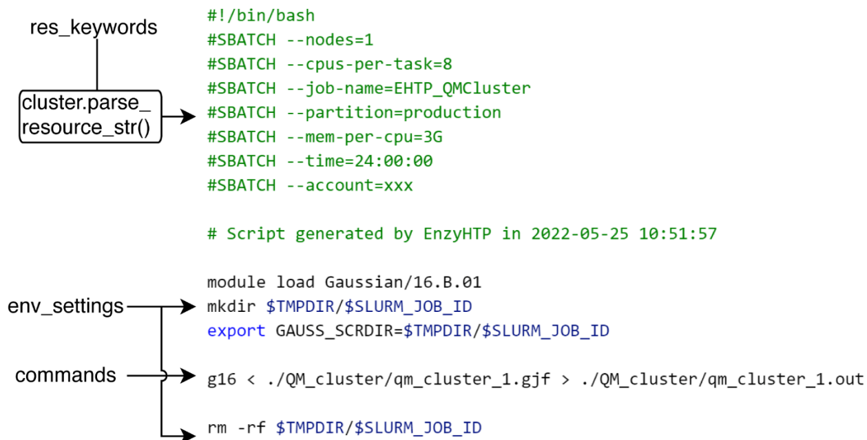
Figure 3. A sample job script that performs QM calculation using Gaussian 16. The job script is generated by the “workflow script” using commands implemented in ARMer.
