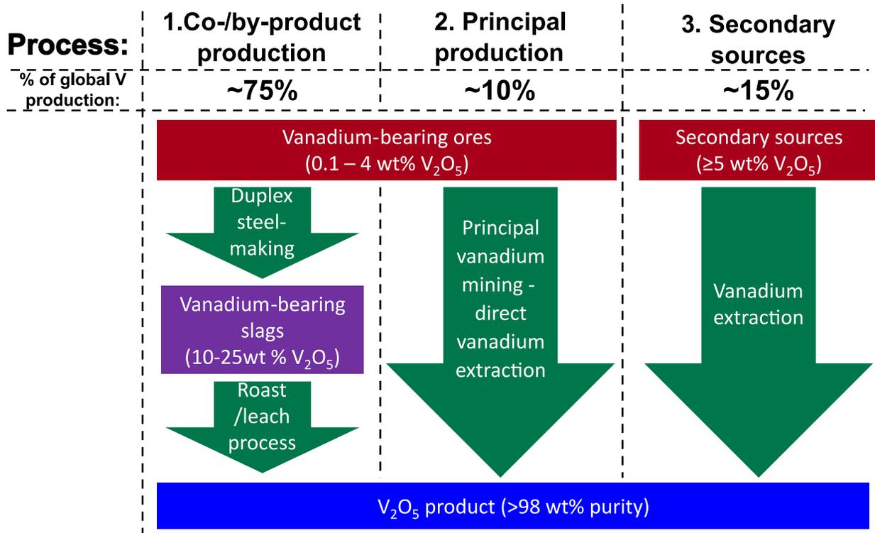
**Figure 3** – Schematic of the three main production routes for vanadium pentoxide ( $V_2O_5$ ).
