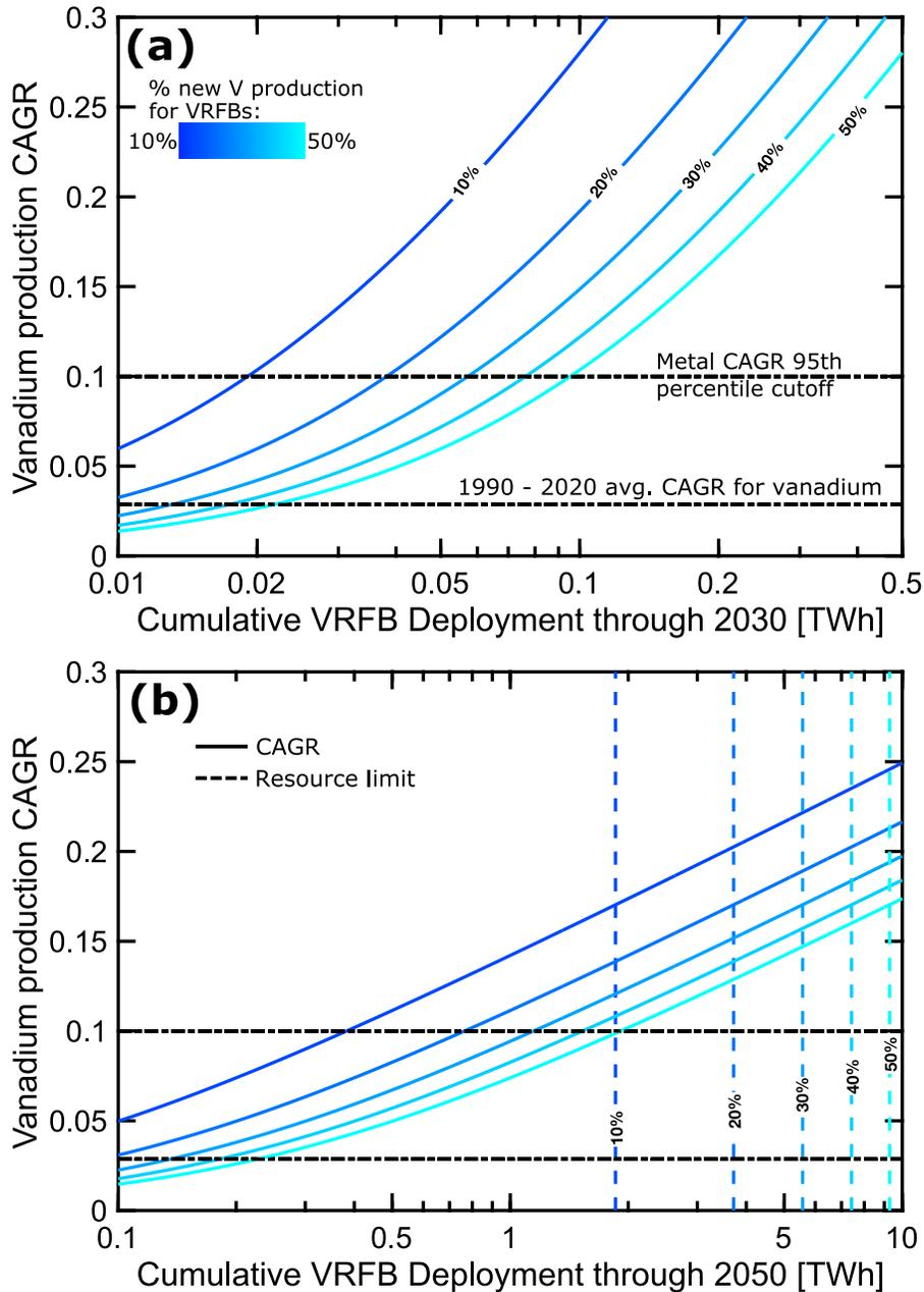
**Figure 3** – Compound annual growth rate (CAGR) of vanadium production needed to achieve various amounts of cumulative VRFB deployment by 2030 (a) and 2050 (b), relative to 2020, based on various scenarios of new fractional production routed to VRFB production over other applications (various shades of blue). The 2050 plot also shows the resource limit under each scenario (vertical dashed lines). The black horizontal lines show relevant historical CAGRs.
