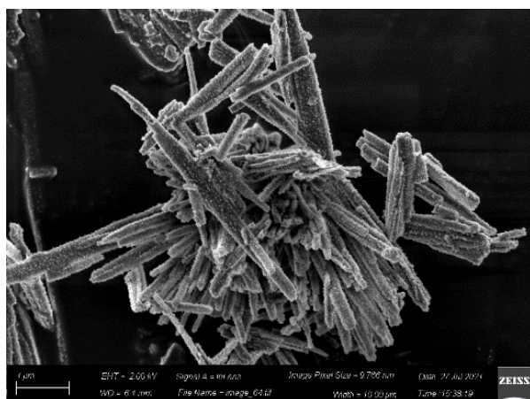
Figure S37. SEM images of \text{Ni}_2\text{Cl}_2(\text{btdd}) prepared under ionothermal conditions.
