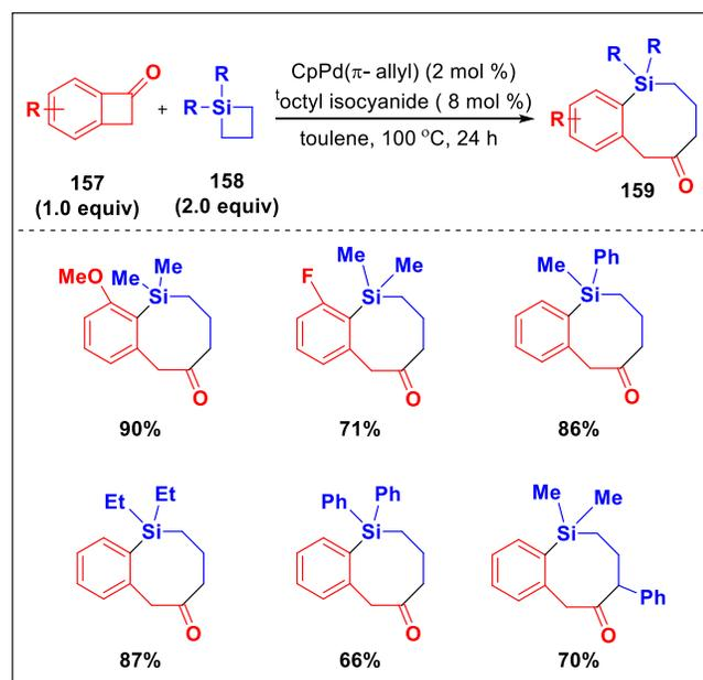
Scheme 6.4 Palladium-catalyzed intermolecular exchange between C-C and C-Si  $\sigma$ -bonds.
