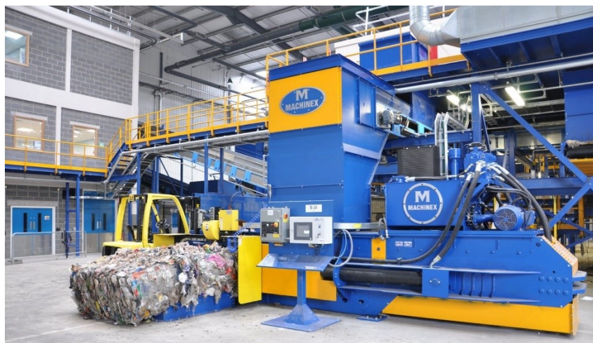
Figure 13. Two-ram Baler from Machinex Recycling. Published with permission from ref 108 . Copyright Machinex Technologies.
