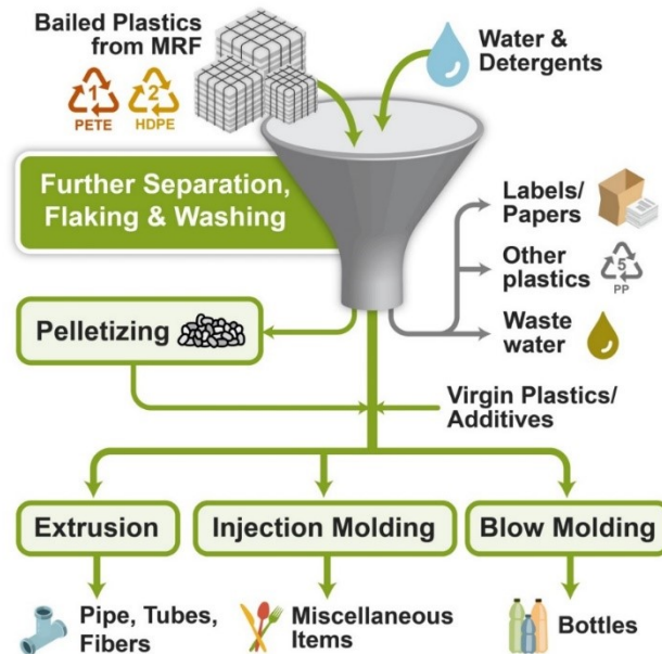
Figure 15. Various approaches for mechanical recycling of PSW (Plastic solid waste). 138
