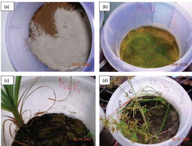
Figure 1. (a) Mount Talang's tephra applied on the surface of soil; (b) surface of tephra layer after 4 months; (c) surface of the 2.5 cm tephra layer after 16 months; (d) surface of the 5.0 cm tephra layer after 18 months. (Reproduced from Ref.25, with kind permission).
