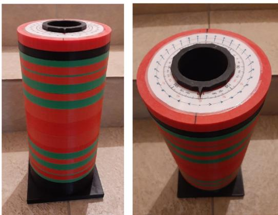
**Figure S10. Magnet used for upper range polarization transfer field variation experiments.** Magnetic fields used to facilitate transfer of polarization to SABRE substrate above the range of ~25 mT were probed using a variable Hallbach array of magnets designed by Dr. Prof. Peter Blümler.
