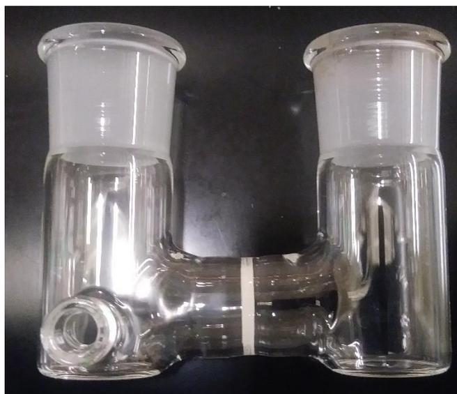
Figure S1. Photo of H-cell used in electrochemical experiments. Custom cell by JamesGlass.
