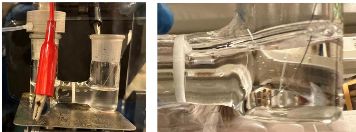
Figure S26. Phase separation observed in anolyte of H-cell during HER at high- $a_{\text{H}_2\text{O}}$  conditions.
