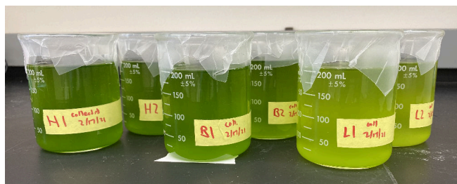
Figure 7. All samples are harvested. 200 mL of algae suspension placed in 250 mL beakers.
