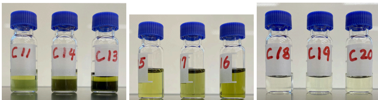
(a) Transesterified samples stored in 1.5 mL GC vials. Pictured are samples after performing hexane extraction, which produced transparent upper layer of hexane. The translucent bottom layer contains a mixture of FAMES and glycerol. C11-L1 Sample; C14-B1; C13-H1.
