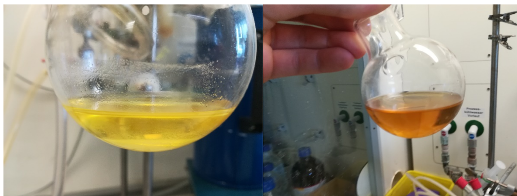
Figure S1. Left: \text{MnCl}_2 \cdot 2\text{LiCl} furnishing high yields in transmetalation. Right: Ate complex with likely impurities of \text{MnCl}_2 leading to low yields in transmetalation.
