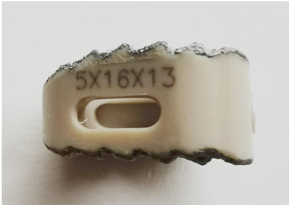
Fig. 1 PEEK cage coated with Ti and HA.
