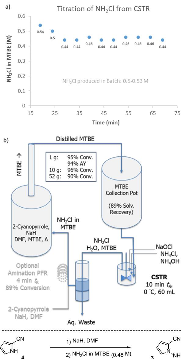
**Figure 5:** Steady state operation of chloramine CSTR and schematic for chloramine generator.
