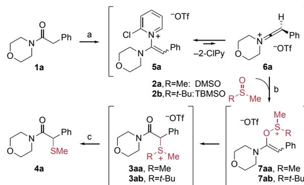
Reagents and conditions: (a)  $\text{ Tf}_2\text{O}$  (1.05 equiv), 2-CIPy (3.00 equiv),  $\text{ CH}_2\text{Cl}_2$ ,  $-78^\circ\text{C} \rightarrow 0^\circ\text{C}$ , 15 min; (b) Sulfoxide (**2**, 1.20 equiv),  $\text{ CH}_2\text{Cl}_2$ ,  $-78^\circ\text{C} \rightarrow 22^\circ\text{C}$ , 45 min; for **3aa**: (c)  $\text{ Et}_3\text{N}$  (10 equiv),  $\text{ MeCN}$ ,  $60^\circ\text{C}$ , 15 h.
