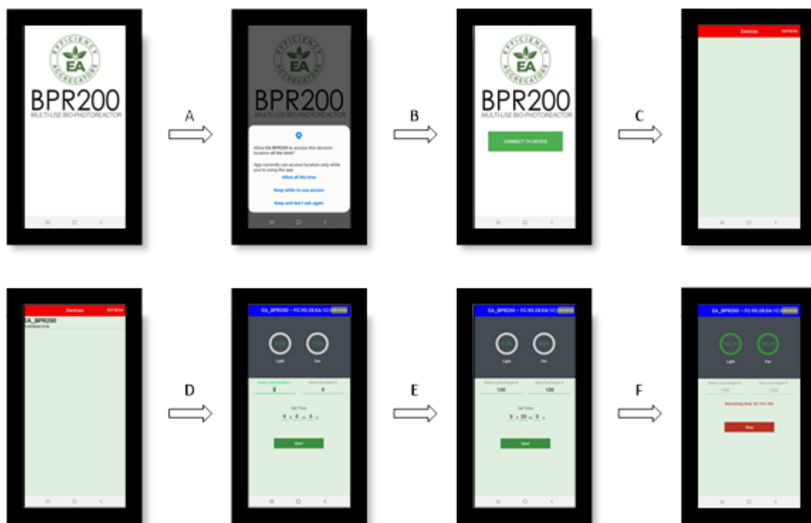
Figure S9. Photoreactor control tablet and instructions on how to turn on the photoreactor. A) Opening the BPR app for the first time will launch a screen asking for various permissions. B) Upon making a choice, the main screen will be displayed. C) Click connect device and the device management screen will pop up. If the photoreactor is plugged in and on, its name should appear on screen after hitting the refresh button. D) Selecting the photoreactor will launch the control screen. E) Input the chosen fan and light intensity and select a reaction time. F) Hit start and irradiation will begin.
