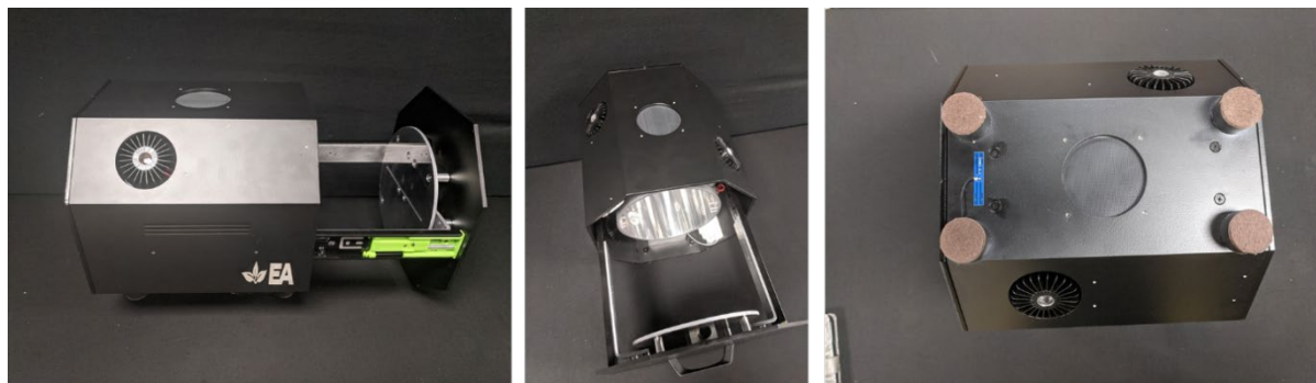
Figure S6: Left, side view of photoreactor outer chamber with lid open. Middle, top view of photoreactor with lid open. Right, bottom view of photoreactor.
