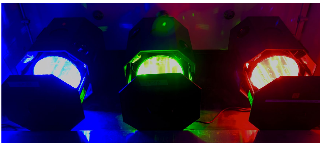
Figure S10: Light on Photoreactor for various wavelengths: Blue ( \lambda=453\text{nm} ), Green ( \lambda=555\text{nm} ), and Red ( \lambda=660\text{nm} ).
