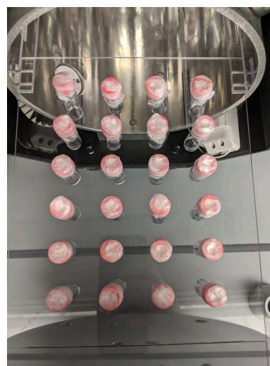
Figure S4: Left, table showing percent conversion at each position in the photoreactor. Right, image of reaction tray to highlight positioning of each vial.
