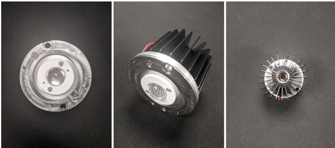
Figure S8: Left, front view of LED Chip. Middle, side view of LED chip showing attached heat sink. Right, back view of LED chip showing heat sink core and fin.
