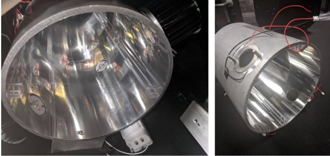
Figure S7: Left, photoreactor inner chamber with reflective interior. Right, outside of inner chamber showing contact pins where LED chips connect.
