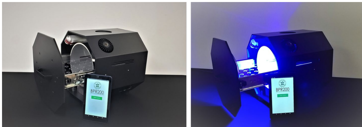
Figure S5: Left, side view of photoreactor with control tablet (light off). Right, side view of photoreactor with control tablet (light on).
