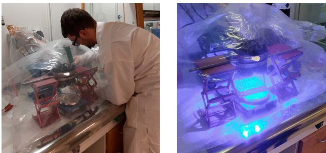
**Figure S9.** a) photo showing the removal of the plate lid within the CO<sub>2</sub> glove-bag for mass screening of substrates. b) 96 well plate reactions running in the CO<sub>2</sub> glove-bag set up.
