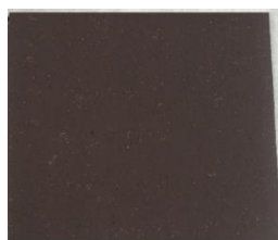
Figure S3. Digital image of Cu deposited on a gas-diffusion electrode.
