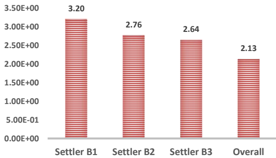
Graph 4. Partition coefficients of trimetozine in the different settlers of the LLE platform and the overall extraction distribution.
