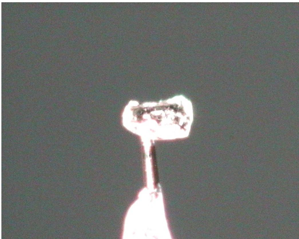
A single crystal of the compound mounted on a glass fiber.
