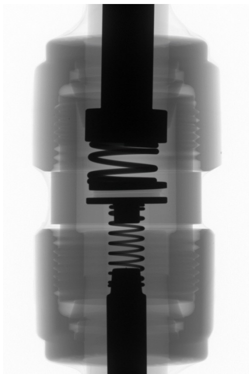
Figure S5: X-ray tomography image showing a sectional view through the center of the applied cell setup with outer current collector, stainless steel spring, stainless steel current collector, battery stack (sodium metal, separator layers, sodium metal), stainless steel current collector, stainless steel spring, outer current collector (from top to bottom); battery housing made of PTFE surrounding the interior.
