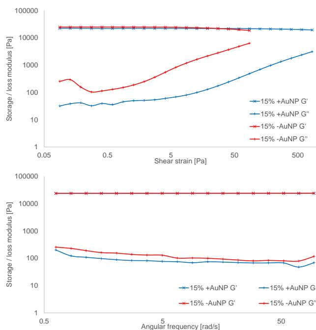
**Figure 3.** Comparison of rheology of gels with (+AuNP) and without (-AuNP) gold nanoparticles. Strain sweep (top) and frequency sweep (bottom) of 15 % PA gel. In the lower graph the two  $G'$  curves follow nearly exactly the same path.
