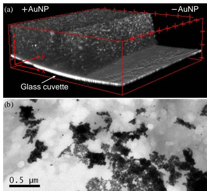
**Figure 4.** (a) OCT volume illustrating inhomogeneity of +AuNP layer compared with that of the pure acrylamide (-AuNP) layer (scan of  $1.5 \text{ mm} \times 1.5 \text{ mm}$  lateral  $\times 1.5 \text{ mm}$ , measured in air). (b) TEM image of DMAP AuNPs forming large aggregates within the PA gel matrix.
