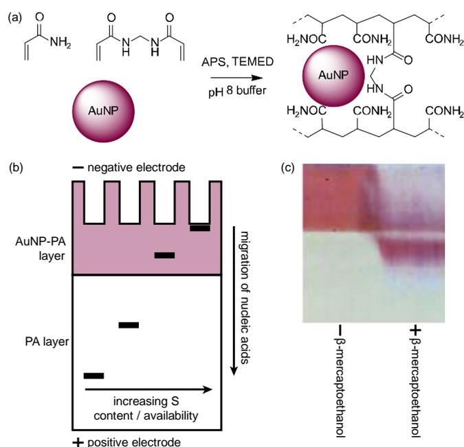
**Figure 1.** (a) Polymerisation of acrylamide and bisacrylamide to give crosslinked gels containing AuNPs. APS = ammonium persulphate; TEMED = tetramethylethylenediamine. (b) Resultant architecture of gel slabs for electrophoresis and expected alterations in migration according to sulphurous functionality. (c) Image of gel contain citrate AuNPs run in the absence and presence of excess thiol.
