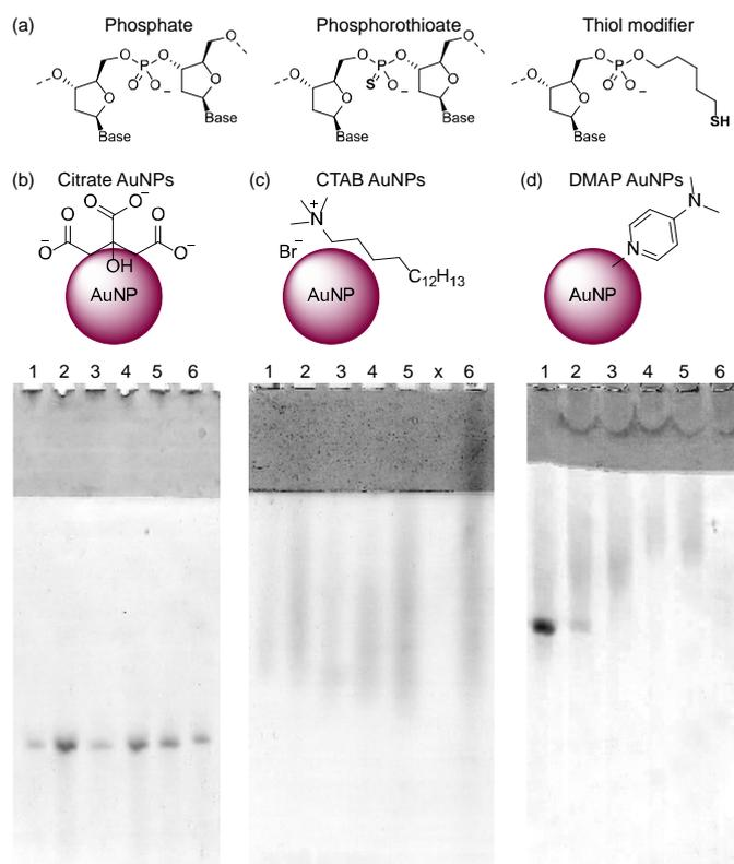
**Figure 2.** (a) Sulphur-modified DNA used herein. (b-d) Gold-PAGE using three types of AuNP. Lanes: 1 = **0S**; 2 = **1S-term**; 3 = **1S-cent**; 4 = **2S**; 5 = **3S**; 6 = **SH**; x = unused. All gels run under denaturing conditions (urea) in TBE buffer at room temperature. (b) Citrate AuNPs (1 mg Au mL<sup>-1</sup>) in 8% PAGE. (c) CTAB AuNPs (1 mg Au mL<sup>-1</sup>) in 8% PAGE. (d) DMAP AuNPs (10 mg Au mL<sup>-1</sup>) in 12% PAGE.
